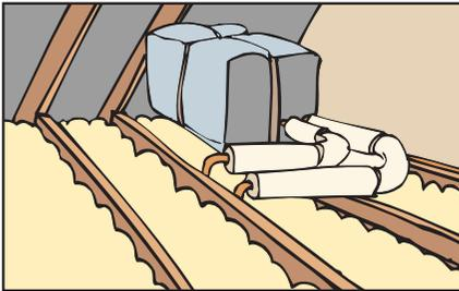
Put strips of insulation around hot water pipes and the hot water tank and on the floor of the loft.
